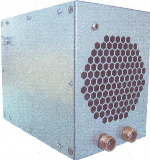
Compact air / water unit with fan for heating or air cooling applications. Maximum heating performance – 1.7kW (US 5800BTU/h). It is equipped with an air condensate drain for use in a geothermal - heat exchanger cooling system without the use of a heat pump.
